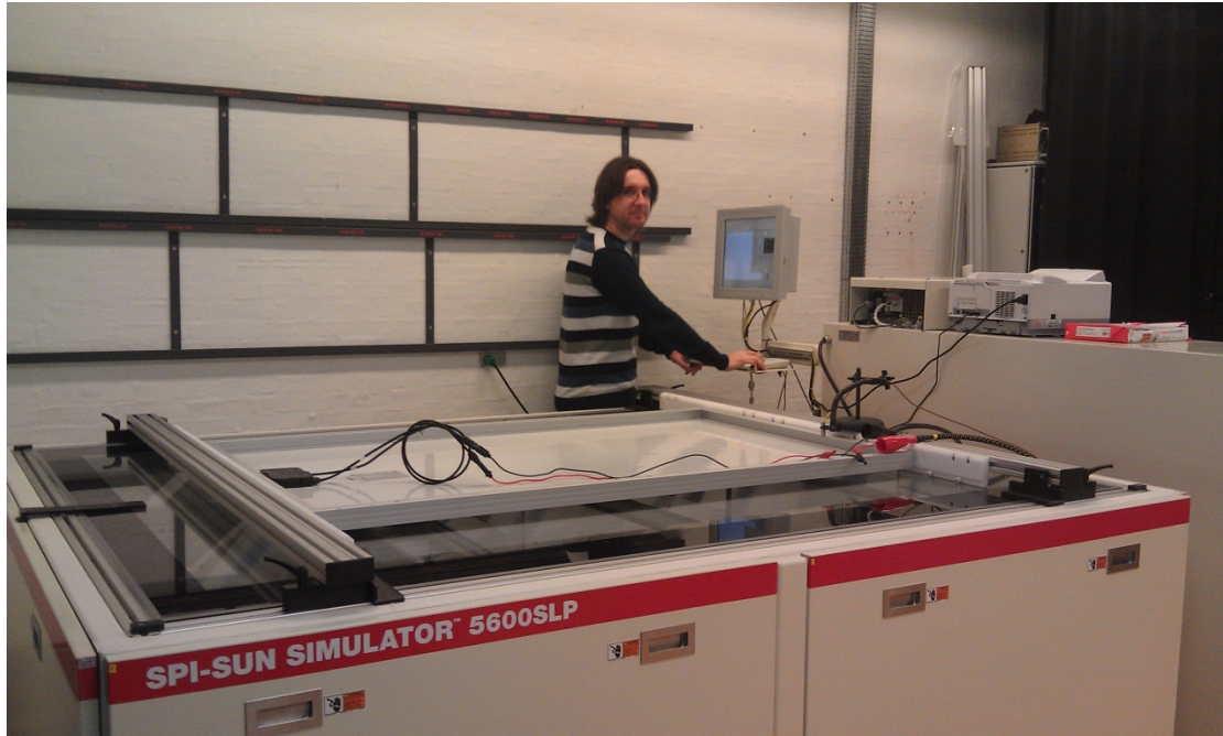
Fig. 2-2 Photo of the Spi-Sun 5600 SLP with a PV module under test
